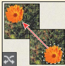
The Content-Aware Move tool recomposes and blends pixels to accommodate a moved object.
